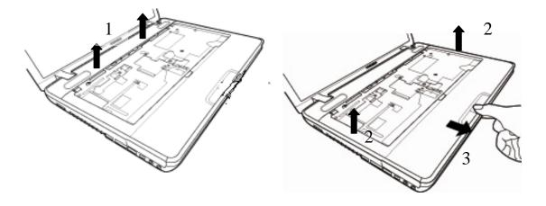
Figure 4-17 Removing top cover
